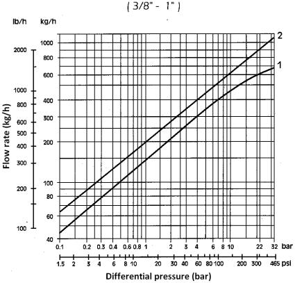
Curve 1: discharge 10 °C below the saturated curve Curve 2: discharge 20 °C below the saturated curve
